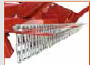
Chains provide safety from thrown objects
