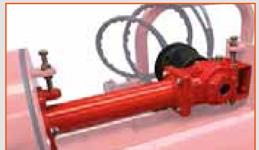
Manual belt tensioning
