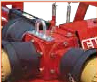
Heavy duty center-splitter gearbox
