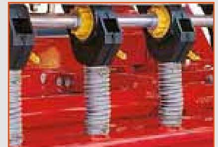
Precise seed metering cups
