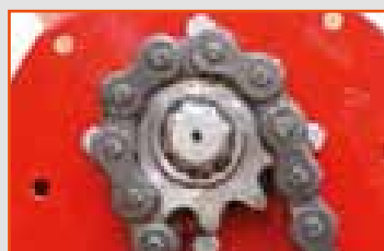
Lateral ASA 60 chain drive transmission in oil bath
