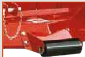
Standard front antiscalping roller
