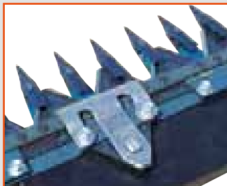
Spring loaded blade guides for quick and easy blade replacement
