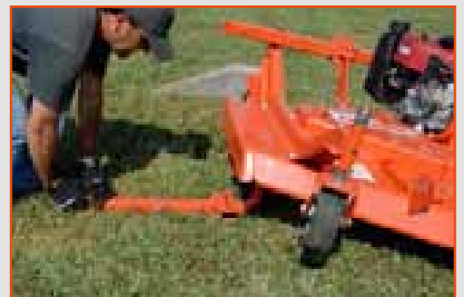
Height adjustment bar
